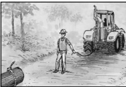
c. Enganche del cable principal
